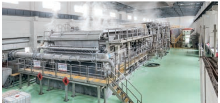
▲ ANDRITZ's delivery of the pulp drying plant (1,200 admt/d of kraft or 950 admt/d of dissolving pulp) has some advanced and innovative energy-saving technologies to reduce operating costs.
