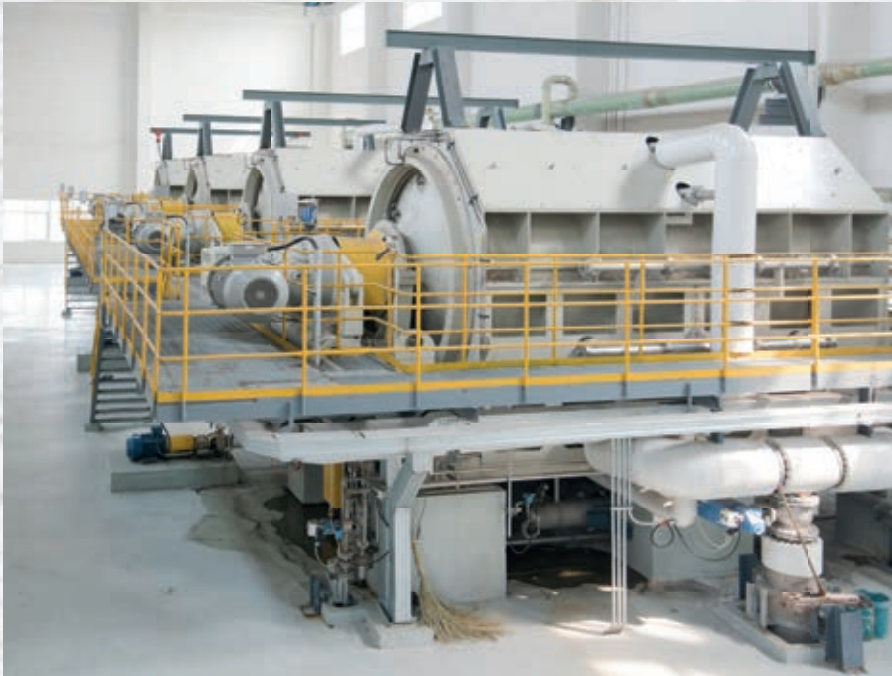
▲ Following the new continuous digester are multi-stage DD Washers for brownstock washing and post-oxygen washing, and a single-stage DD washer after every bleaching stage.
