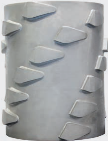
▲ Figure 4. DRUM 450 Dolphin rotor for coarse screening. The rotor creates optimal pressure pulses (positive pulse for debris removal efficiency and negative pulse for cleaning to minimize plugging).
