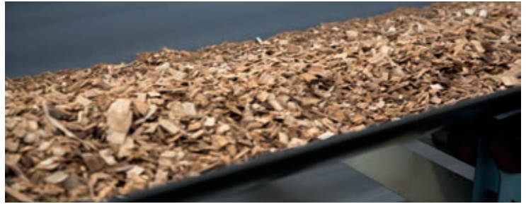
▲ ANDRITZ provided the basic engineering and chip screening technology ensuring that incoming chips are of optimum size for the cooking plant. Oversized chips are treated in a new ANDRITZ rechipper.
