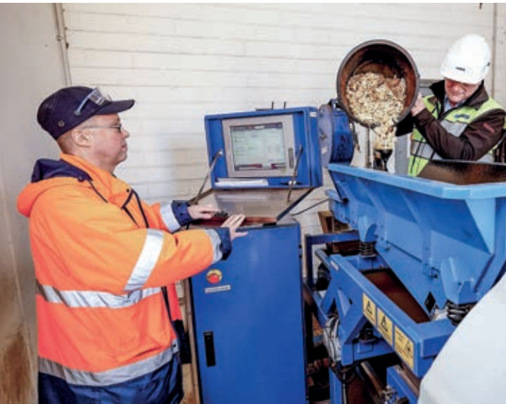
▲ The ANDRITZ ScanChip analyzer monitors chip quality and helps the mill determine the optimum time for chipper knife changes. Josef Ertl, ANDRITZ Product Manager (right), pours chips into the analyzer as Steffan Ratzlow, Zellstoff Stendal's Fiberline Manager, looks on.
