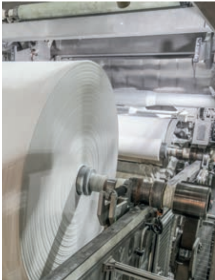
▲ Tissue on the reel – TM1 produces heavy weight toilet tissue; TM2 produces lighter weight toilet tissue and facial tissue.
