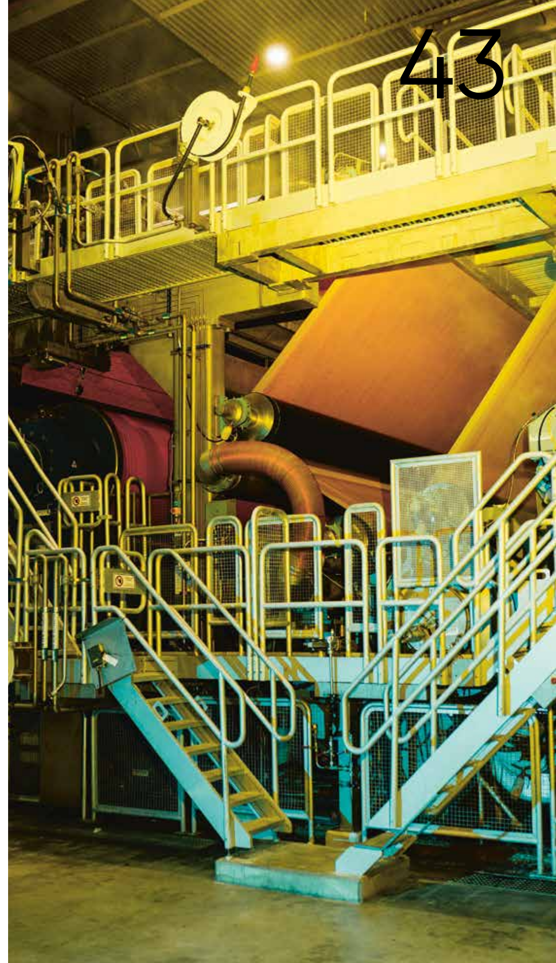
EvoDry™ pulp drying system from ANDRITZ with energy-saving technologies that reduce the mill's operating costs significantly. The system includes energy recovery from the boiler waste heat, fine screening, and a twin wire dewatering system with fully automatic tail threading that meets the strictest health, safety, and environmental regulations.
