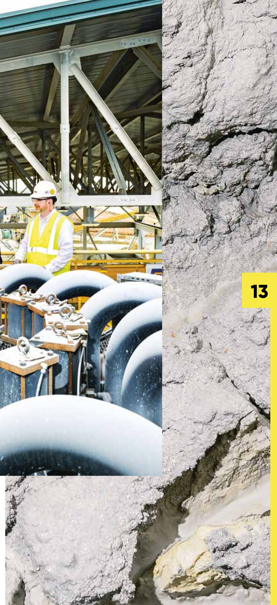
Anderson and Schug at one of the grinding area hydrocyclones where the ore undergoes beneficiation in a physicochemical process.
