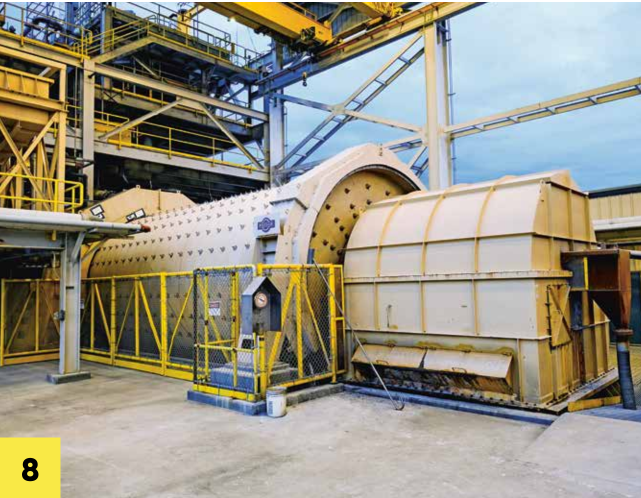
The drum of the ball mill is as big as a house. It rotates around its own axis in just a few seconds.
