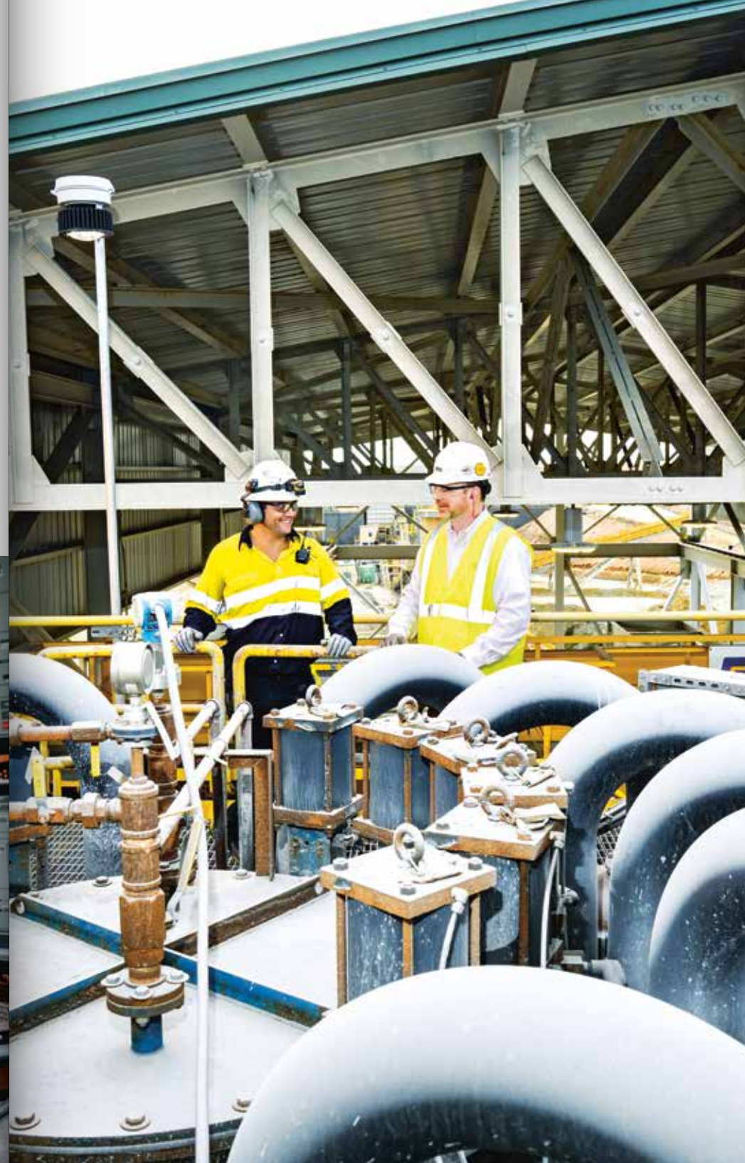
Anderson and Schug at one of the grinding area hydrocyclones where the ore undergoes beneficiation in a physicochemical process.
