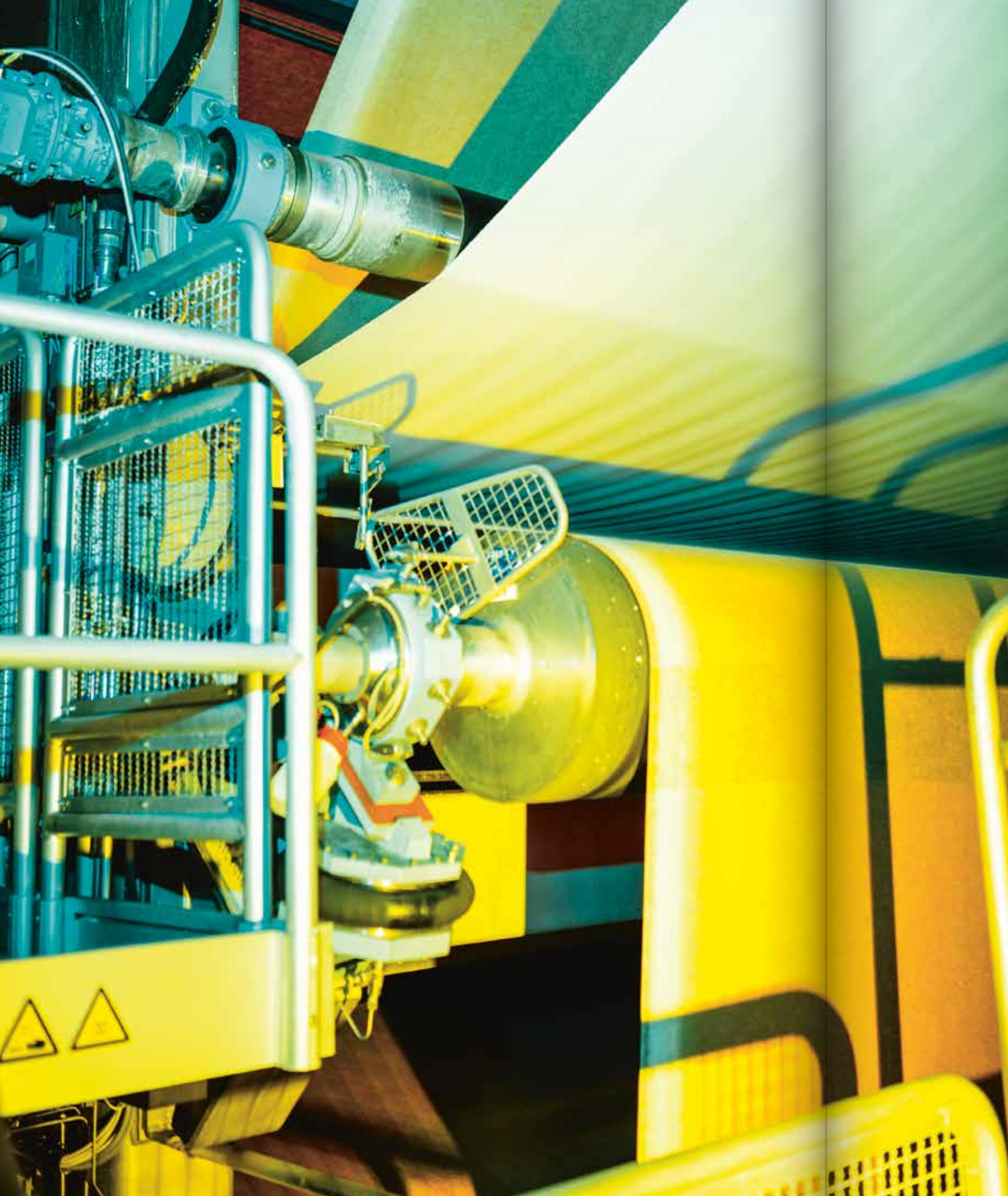
EvoDry™ pulp drying system from ANDRITZ with energy-saving technologies that reduce the mill's operating costs significantly. The system includes energy recovery from the boiler waste heat, fine screening, and a twin wire dewatering system with fully automatic tail threading that meets the strictest health, safety, and environmental regulations.
